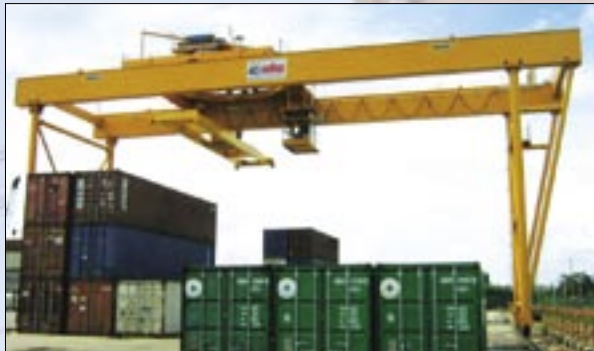
A 40 t portal crane equipped with spreader for container handling, Malaysia
