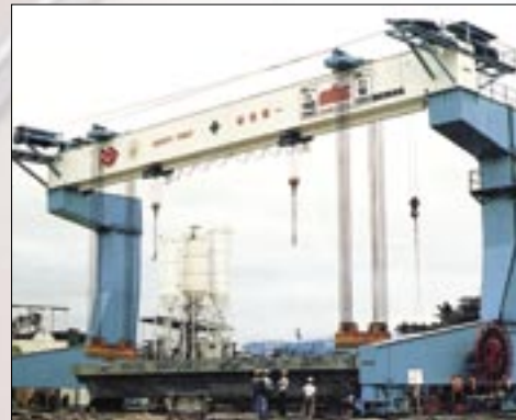
A 2 x 140t / 10t C-shaped gantry crane designed for special application in a pre-fabrication yard for Singapore Mass Rapid Transit Project.
