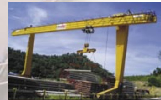
A C-shape crane with a load attachment to handle concrete beams.
