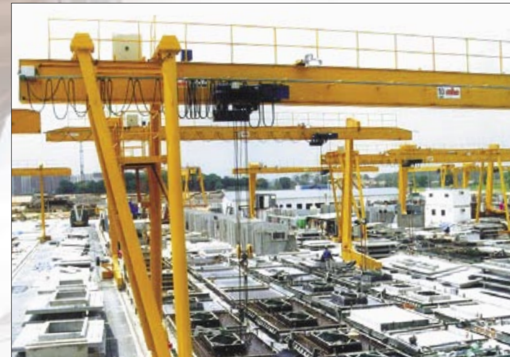
Single girder portal cranes designed for handling concrete slabs in a prefabrication yard.
