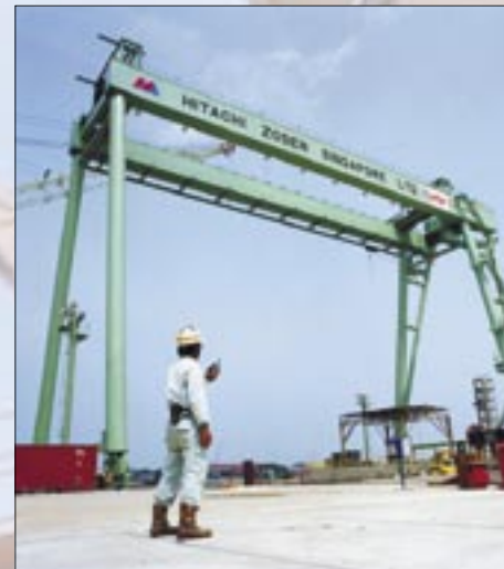
A full portal crane with a span of 60m and SWL of 100t in a shipyard.
