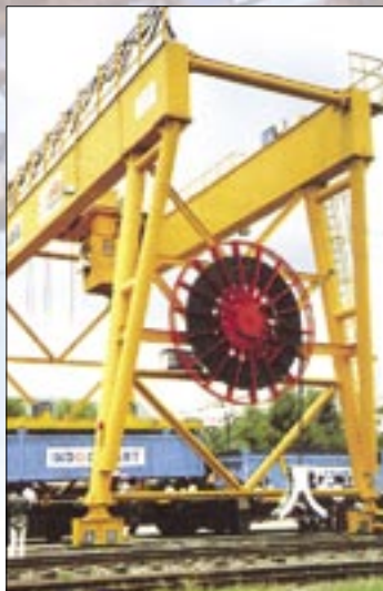
A full portal container handling crane with motorised cable reels in operation in a coal terminal in Indonesia.
