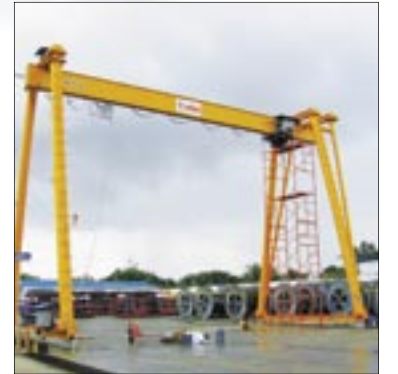
A 10t x 12m span full-portal crane handling and storing cable drums in a stockyard.
