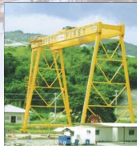
An 80T crane used to manufacture pipes for a hydroelectric power station.
