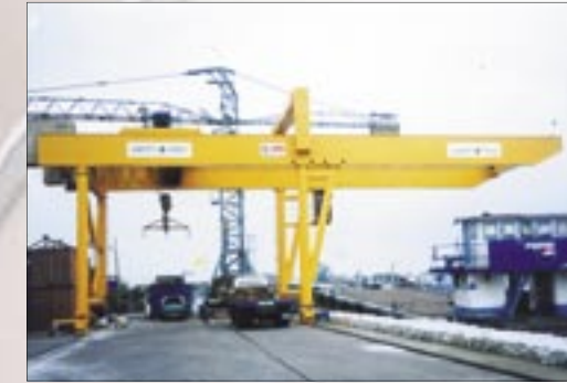
A full portal crane with an extended cantilever arm to load and unload materials onto barges.
