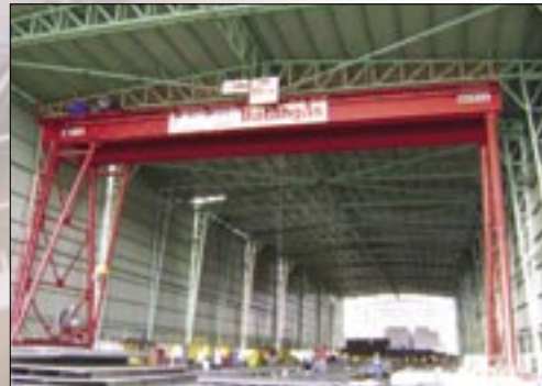
A 20t full portal crane used for ship fabrication and repair, Philippines.
