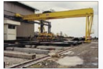
A semi-portal crane using magnets to handle metal plates.
